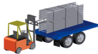
Figure 1b Incorrect method of removal
